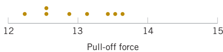
FIGURE 1-2 Dot diagram of the pull-off force data when wall thickness is 3/32 inch.
